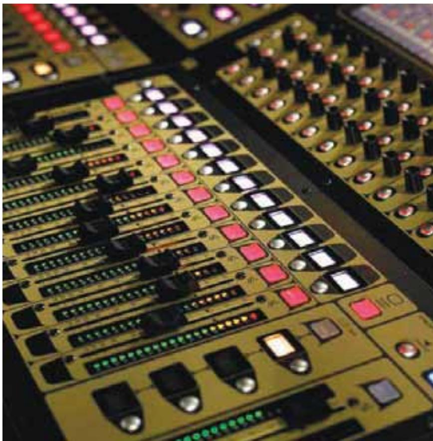
allowing all 36 main faders to control inputs if desired, while any bank of 12 can be assigned to the touch screen for fine-tuning. The SD8 provides, as standard, a 12 x 12 output matrix, its 12 busses being additional to the console's 24 stereo, solo and master busses.
